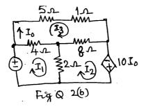
c. Calculate the current through 2  $\Omega$  resistor in the circuit of Fig. Q2(c) using source information.
