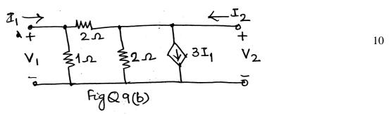
10a. For the network shown in Fig. 10(a) compute  $\alpha_{12}(s) = \frac{I_2(s)}{I_1(s)}$  and  $Z_{12}(s) = \frac{V_2(s)}{I_1(s)}$ . Also locate
