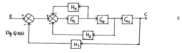
c. Obtain the closed loop transfer function  $\frac{C(S)}{R(S)}$  by using Marson's gain formula for the signal
