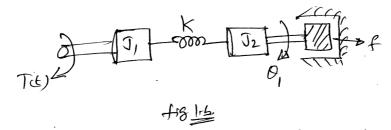
c. For the mechanical system shown in Fig. 1c, obtain force-voltage analogous circuit,
