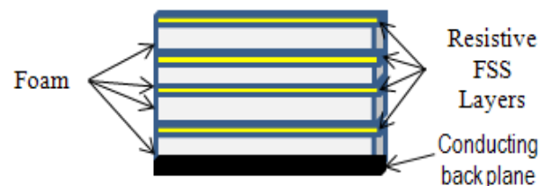
Fig. 1. Dielectric profile of UWB panel RAM.
