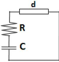
Fig. 2(a). Transmission line equivalent circuit of RAM.
