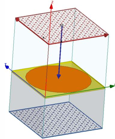
Fig. 3. Unit cell geometry model of RAM in HFSS.
