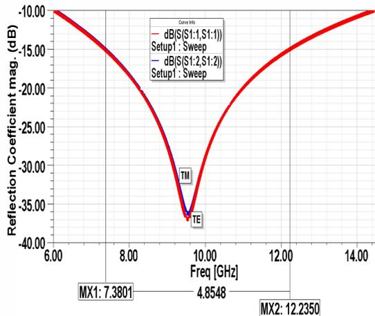
Fig.4.Optimized simulation performance of RAM for circular polarization.
