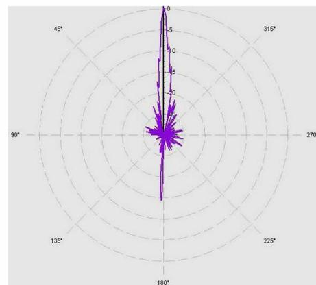
Fig. 7. RCSR plot of panel RAM. Frequency 8 GHz. Polarization: VP . RCSR = 15 dB.
