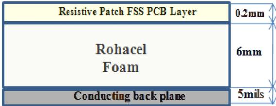
Fig. 1 Dielectric profile of the thin RAM.
