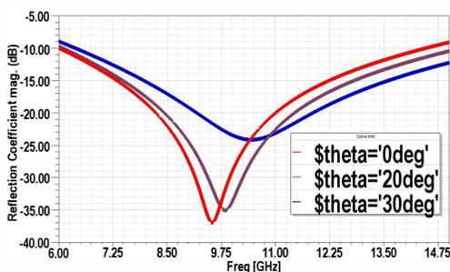
Fig.5.Off-normal incidence simulation performance of RAM.TE incidence.
