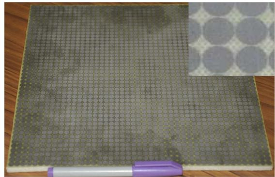
Fig. 6. Photograph of prototype panel RAM. Size: 280 x 280 mm. Thickness = 6.2 mm. Inset: Zoomed cells for clarity.
