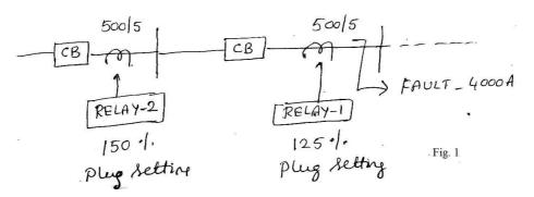
For discrimination, time grading margin is 0.6 s. Determine the time of operation of two relays assuming that both the relays have character as shown in Fig. 2. The relay-1 has time setting multiplier of 0.3. Find the time setting multiplier of relay-2.
