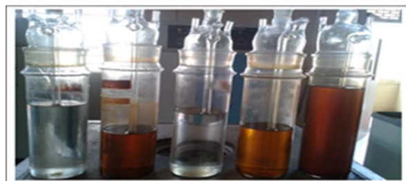
Figure 3. Photograph showing color of oils: (i) before aging (ii) after aging for 384 hours with 193 ppm of DBDS, (iii) aged for 384 hours and extracted, (iv) extracted oil aged for 432 hours and (v) oil aged for 816 hours without extraction (in order from left to right).
