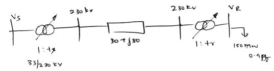
c. Explain voltage control by using Booster Transformer .
