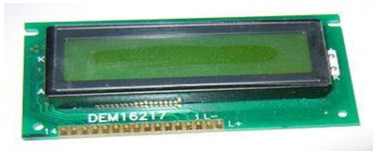
**Fig.2(b): Alphanumeric LCD**
