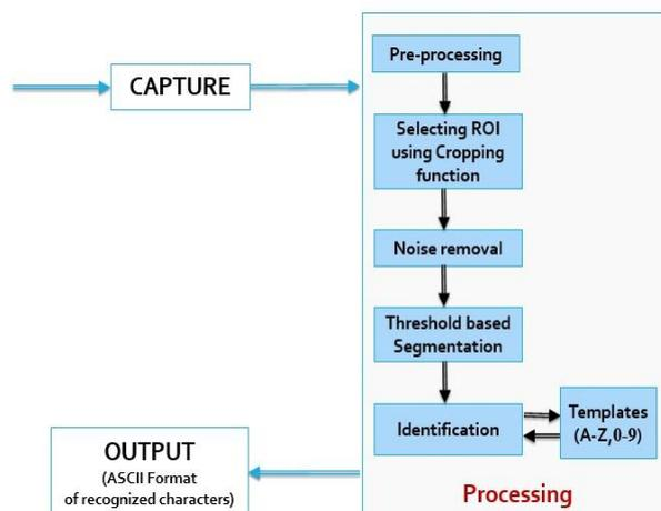
Figure 3: Architecture of the proposed system
