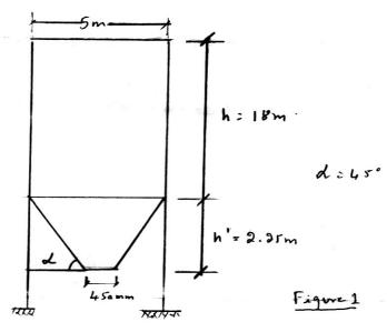
8. A cylindrical silo has an internal diameter of 6 m and 20 m deep (cylindrical portion) with a conical hopper bottom. The material stored is poultry feed having a density of 8 kN/m<sup>3</sup>. The coefficient of friction between wall and material is 0.444. The ratio of horizontal to vertical pressure intensity is 0.40 angle of repose = 25°. Design the reinforcements in the silo walls. Adopt M20 grade concrete and Fe 415 steel. Adopt Janssen's theory for pressure calculation.
