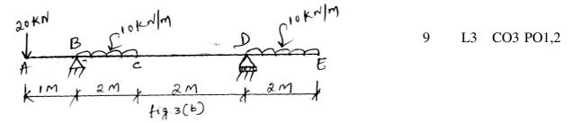
c. Draw BMD and SFD for the beam shown in Fig. 3(c). Find the point of contra flexure if any.
