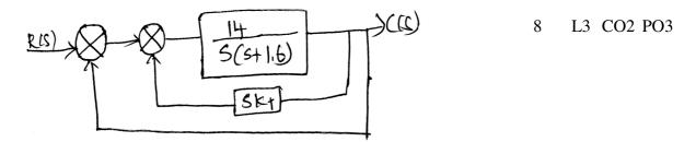
c. For the control system shown below, what is the value of *K* for the system to be critically damped?
