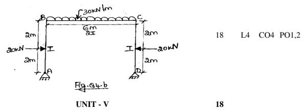
5 a. Analyze the portal frame loaded as shown in Fig. Q5a. Using flexibility matrix method, draw BMD and elastic curve. Take EI as constant.
