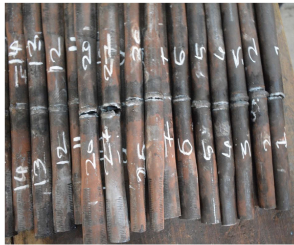
Fig.2: Failure of the specimens
