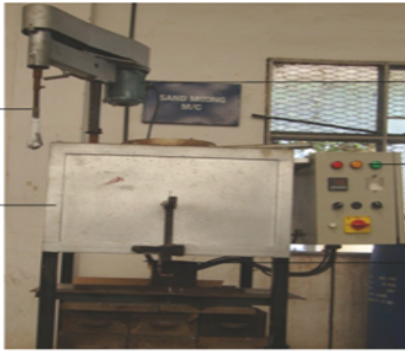
Fig. 1: Electrical Heating Furnace
