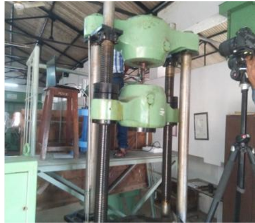
Fig 2. Tensile Experimental Setup
