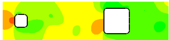
Fig.7 Pressure distribution plot for two square cylinders with chamfered and rounded at the corner of different size when PPR is 6 for Re=200.
